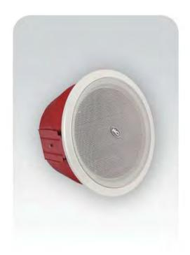
The metal grille, metal baffle and fire dome metal back can plus ceramic connector, thermal fuse and fire-resistant cable, all of the above features make it is fireproof. Its spring clamp type makes the easy and secure installation.
